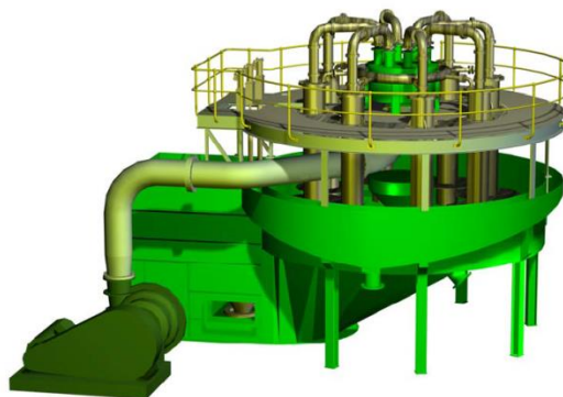
Figure 16: Schematic of a Jameson cell (Z Cell type) Source: (Cowburn, et al., 2005)
