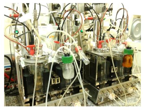
Figure 6.1 Bioreactor Multifors 2 incubated with A. terreus NRRL 1960.
