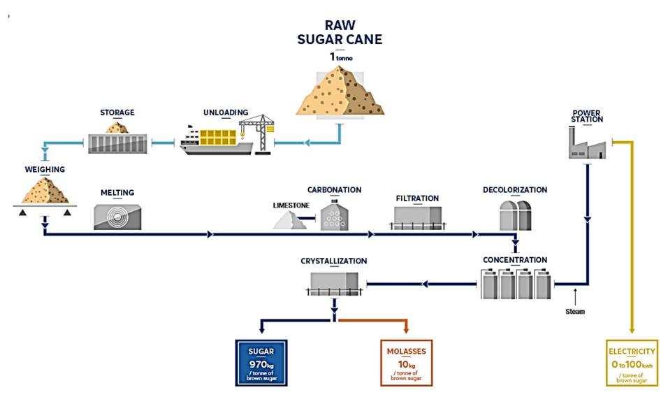
Figure 3.3 Simplified flow diagram of refined sugar, molasse and electricity production at a sugar refinery (SUCDEN 2017a).
