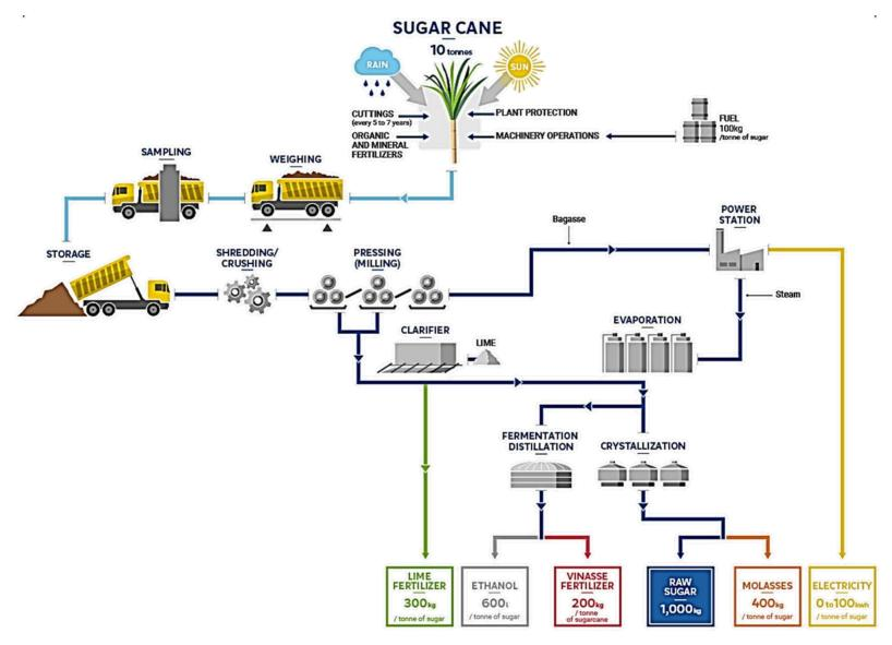
Figure 3.2 Simplified flow diagram of raw sugar, ethanol and electricity production at a sugarcane mill (SUCDEN 2017a).
