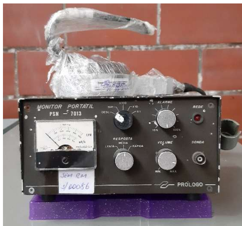
Figure 2.22: Example of Geiger detector model 7013 with pancake probe made in Nuclear Engineering Institute.
