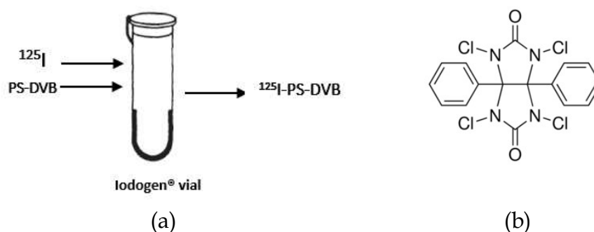
Figure 2.11: Scheme of PS-DVB radioiodination by the Iodogen® method (a). The bottle has the walls lined with the oxidant. The reaction occurred at room temperature. Adapted from Dewanjee (64). Chemical structure of Iodogen®.
